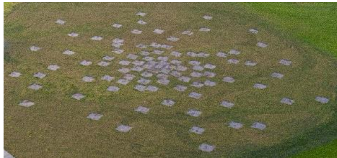
Fig. 1. Aerial view of the Low-Band Antennas (LBAs) of one LOFAR station.
