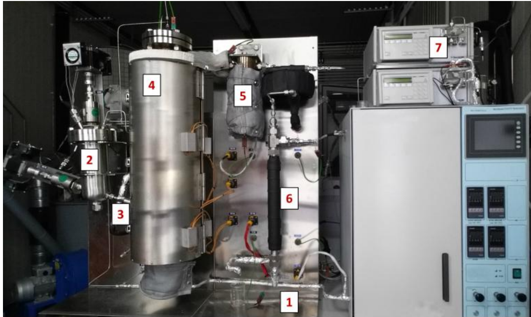
1. INLET FEEDING GAS LINE 4. BUBBLING FLUIDIZED REACTOR 7. HPLC PUMP 2. FEEDING VESSEL 5. CYCLONE 3. FEEDING SCREW 6. TAR COLD CONDENSER
