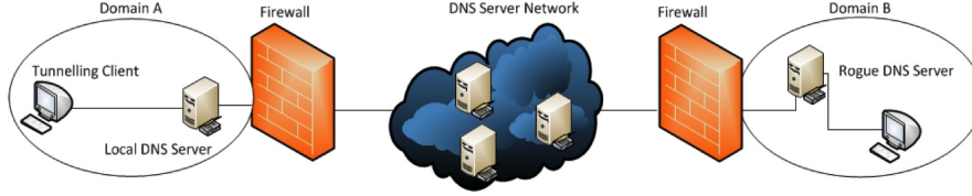
FIG. 1: Entities involved in a DNS Tunnel
