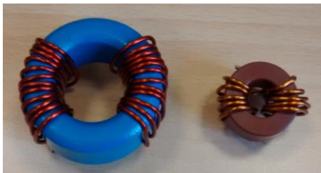
Fig. 9. CM choke set up by using an N30 ferrite core (left) and a VITROPERM core (right).
