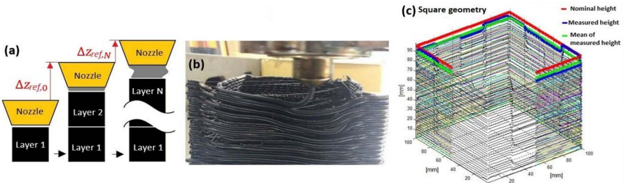
Fig. 6 Robot height above the optimal range: (a) conceptual scheme; (b) deposition experiment; (c) deposition defect measured with laser sensor.
