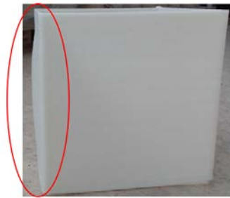
Fig. 10 Dimensional errors on a simple ABS object.
