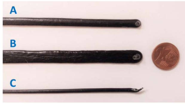
Fig. 3 Examples of PLA deposited tracks at the experimental conditions A: \omega_m = 650 rpm, v_t = 20 mm/s, \Delta z_{ref} = 2.0 mm; B: \omega_m = 900 rpm, v_t = 15 mm/s, \Delta z_{ref} = 1.5 mm; C: \omega_m = 400 rpm, v_t = 25 mm/s, \Delta z_{ref} = 2.5 mm.
