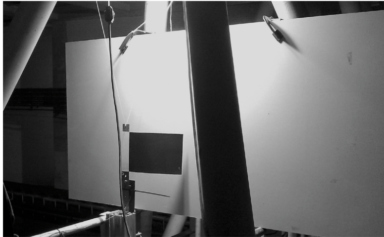
Figure 3: Experimental set-up: test section on the towing-tank carriage.
