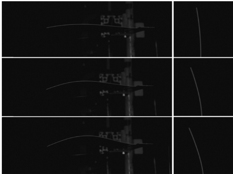
Figure 16: Snapshots of the flag motion for h = \infty and U/U_F = 1.325 (negative image).
