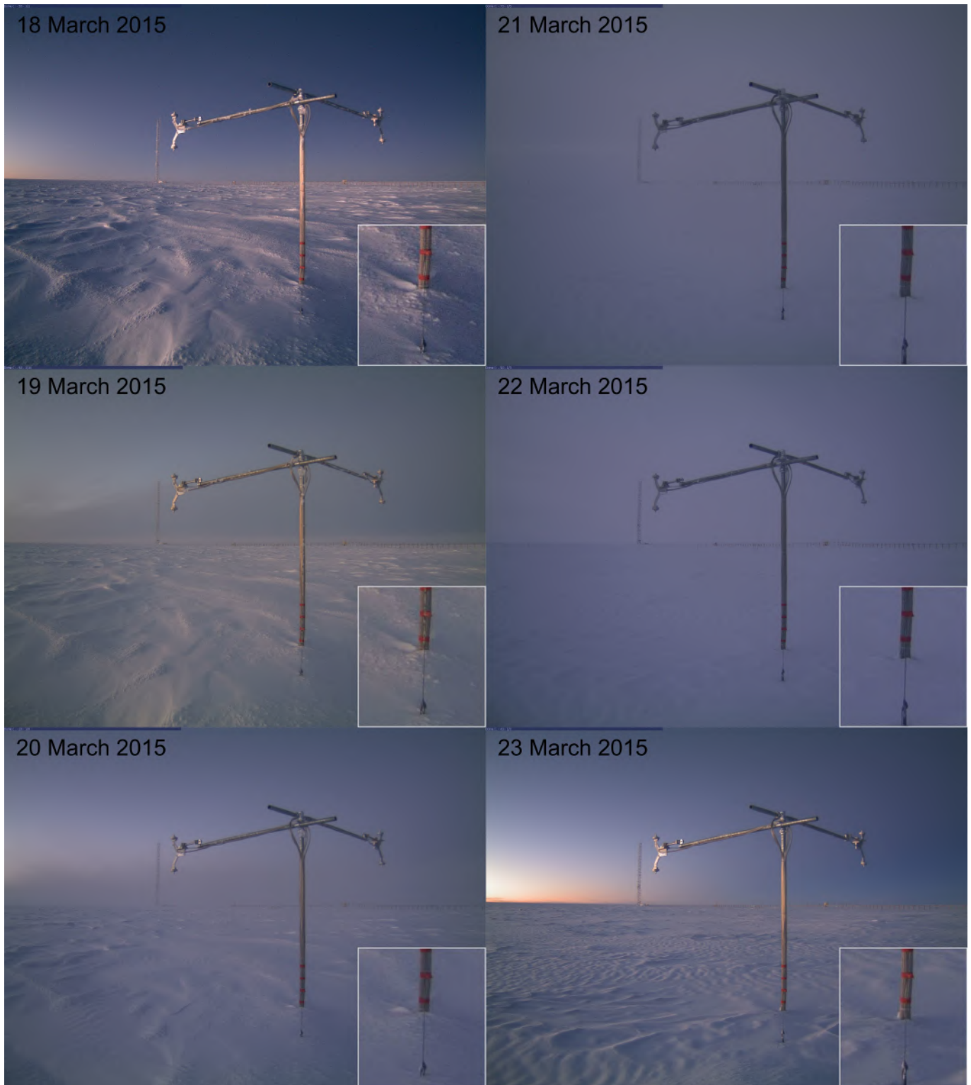
Figure 5: Dome C area photographs from 18 to 23 March 2015 between 10 h and 12 h, with a focus on the base of sensor at the bottom right. Red bands are spaced about 5 cm.
