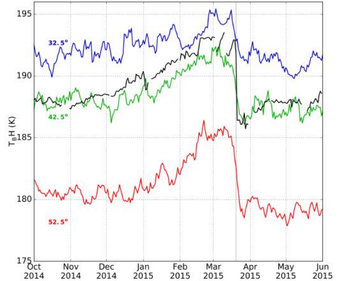
Figure 2: T_B H (K) at Dome C, Antarctica from October 2014 to May 2015 with SMOS at 32.5^\circ (blue), 42.5^\circ (green) and 52.5^\circ (red) incidence angle, and with DOMEX at 42^\circ (black).
